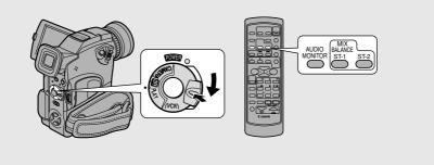
When you play back a tape that was recorded in 12-bit mode, you can set the audio output to play: stereo 1 (the original sound), stereo 2 (any new sound, dubbed to the tape after recording), or mix the balance between the two.
